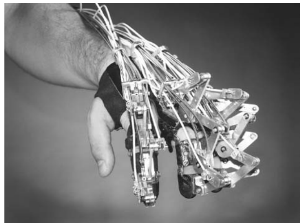
Figure 2 Hand exoskeleton with the mechanics for 16 degrees of freedom (motor unit not shown).
