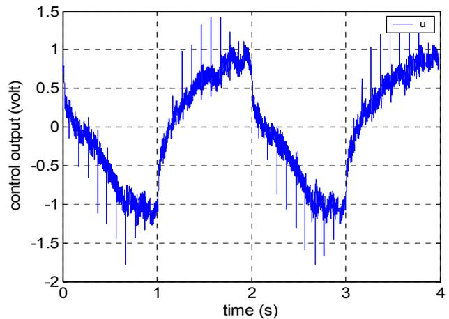
Fig. 8 The control output during execution of the desired trajectory (see Fig. 6). Maximum output voltage was limited to 2 V. The peaks in the control output do not lead to undesired vibrations at the hand exoskeleton.
