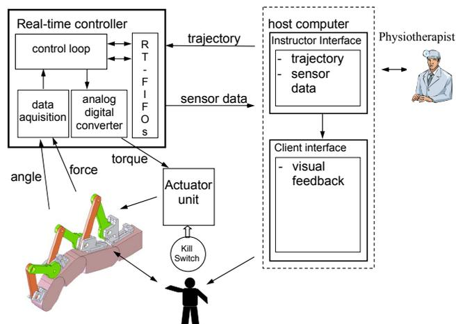
Fig. 2: Diagram of the system. The Real-Time controller samples the sensors data and controls the movement through the actuation unit of the hand exoskeleton worn by the patient. The physiotherapist can supervise the exercises through the instructor interface. The kill switch can abort the movement at any time.
