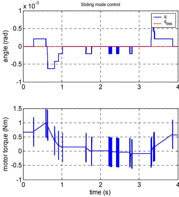
Fig. 5 Error during varying forces holding constant position. Lower Graph shows the varying controller output as a response of the varying forces.
