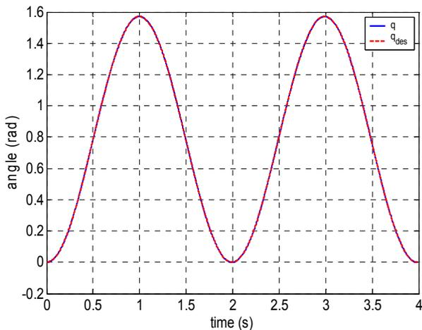
Fig. 6 Desired trajectory (sine wave with a frequency of 0.5 Hz frequency and an amplitude of  $\pi/2$  rad) and actual trajectory for the flexion resp. extension of the MCP.
