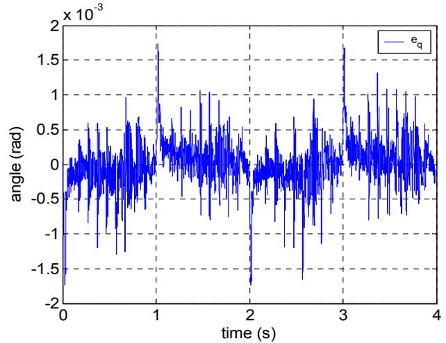
Fig. 7 Position error occurring during execution of desired trajectory (see Fig. 6). The maximum error occur when the direction of the movements is reversed.
