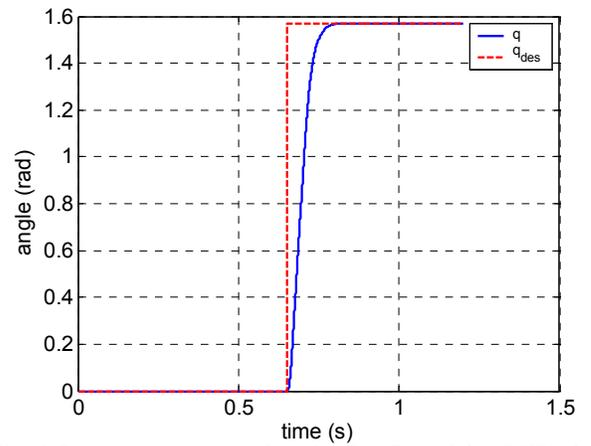
Fig. 4 Step response measured at the first finger joint (MCP) during flexion and extension using the sliding mode control algorithm.
